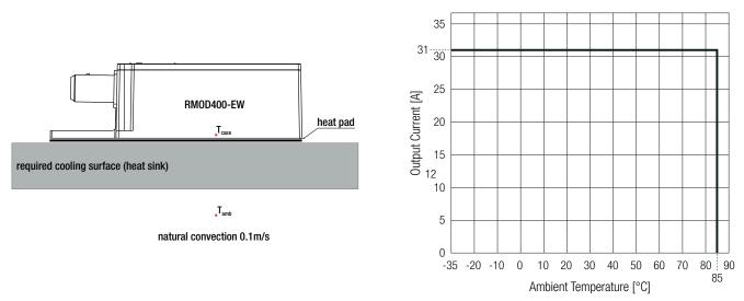
The module can be used in enclosed applications with full load, as long as the cooling is sufficient to keep the baseplate temperature at  $T_{CASE}$  below 70°C. The surrounding temperature should not exceed 85°C.
