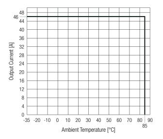
The module can be used in enclosed applications with full load, as long as the cooling is sufficient to keep the baseplate temperature at  $T_{CASE}$  below 70°C. The surrounding temperature should not exceed 85°C.
