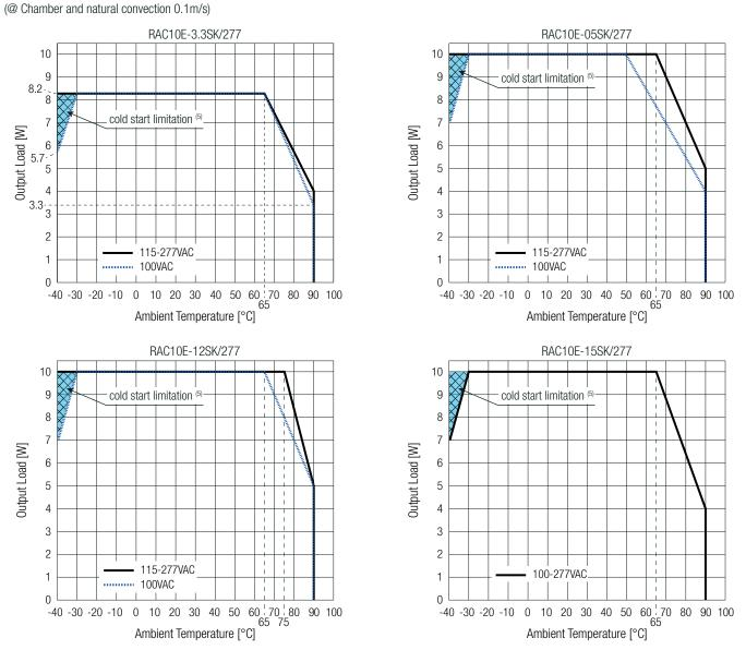
Note5: Cold start is limited to reduced output Power for 15V in general and for 3.3 to 12V versions at use in low line conditions
